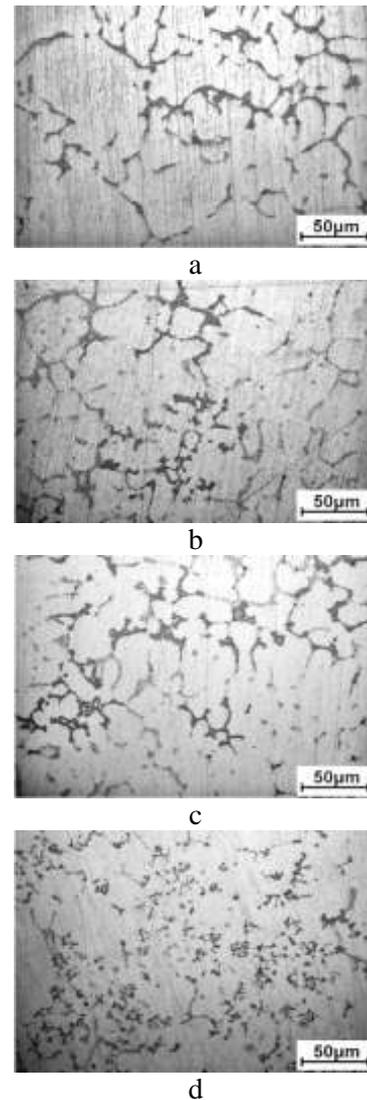
Fig. 3. Microstructure of 2024 alloy after twin-roll casting and heat treatment under different conditions: a – as-cast state; b – HT1 (heat treatment, regime 1); c – HT2; d – HT3
