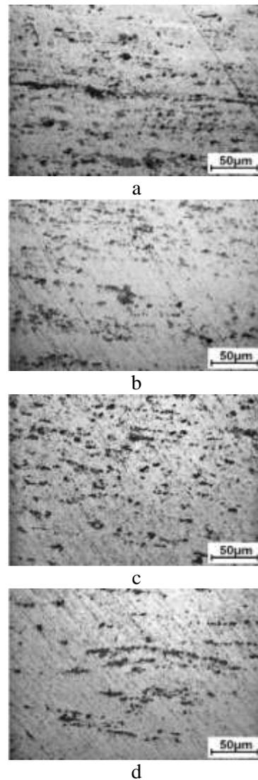
Fig. 5. Microstructure of 2024 alloy depending on the influence of technological factors in the "twin-roll casting + hot rolling ( $\epsilon = 75\%$ ) + heat treatment": a – as-cast + hot rolling; b – as-cast + hot rolling + HT1; c – as-cast + hot rolling + HT2; d – as-cast + hot rolling + HT3
