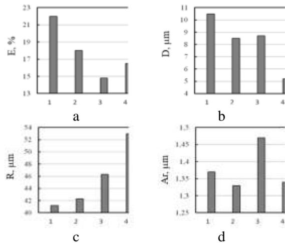
Fig. 4. 2024 alloy quantitative structure characteristics depending on technological factors according to the scheme "twin-roll casting + heat treatment": 1 – As-cast state; 2 – HT1; 3 – HT2; 4 – HT3
