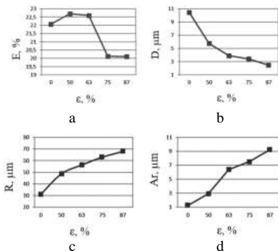
Fig. 2. Quantitative characteristics of the 2024 alloy specimens structure after strip twin-roll casting and hot rolling with various degrees of deformation
