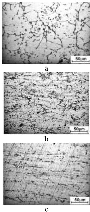
Fig. 1. Microstructure of 2024 alloy after twin-roll casting and hot deformation with different degrees of deformation: a – cast; b –  $\varepsilon = 50\%$ ; c –  $\varepsilon = 87.5\%$
