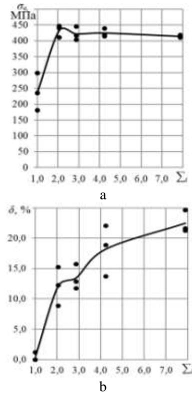
Fig. 7. Experimental data of the dependence of 2024 alloy strip ultimate strength  $\sigma_B$  (a) and relative elongation  $\delta$  (b) on the compression degree  $\Sigma_i$  during hot rolling.
