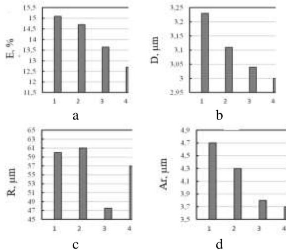
Fig. 6. Quantitative characteristics of the 2024 alloy structure, depending on technological factors in the "twin-roll casting + hot rolling + heat treatment" technological process: 1 – casting + hot rolling; 2 – HT1; 3 – HT2; 4 – HT3
