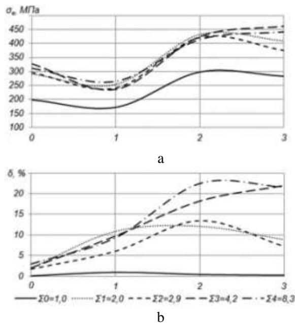
Fig. 8. Effect of heat treatment regimes on ultimate strength (a) and relative elongation (b) of the 2024 alloy strip at different compression degrees  $\Sigma$ : 0 – after hot rolling; 1 – annealing; 2 – quenching with natural aging; 3 – quenching with artificial aging
