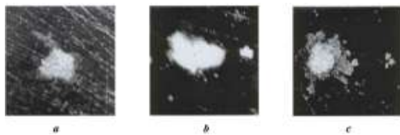
Fig. 5. Traces of singular discharges, obtained for the fixed size of the gap (0.5 mm): a - B=0 T; b - B=0.068 T; c - B=0.086 T. Discharge energy is 0.14 J
